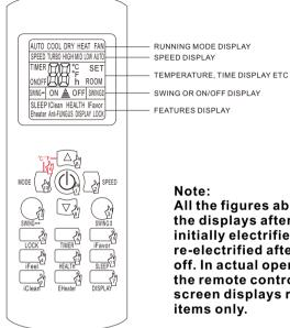
All the figures above are the displays after being initially electrified or re-electrified after power off. In actual operations. the remote controller screen displays related
